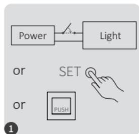
Power off 10 seconds and power on again or short press "SET" one time or turn on light via PUSH switch
