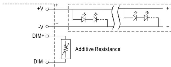
"DO NOT connect "DIM- to -V"
