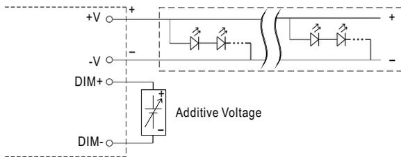
"DO NOT connect "DIM- to -V"
