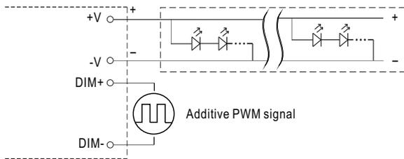
"DO NOT connect "DIM- to -V"
