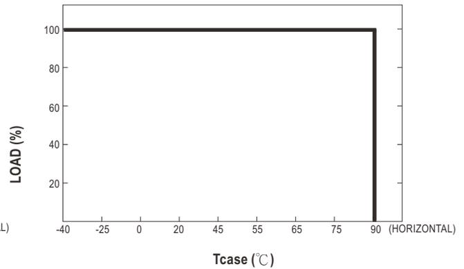
© If HLG-600H operates in constant current mode with the rated current, the maximum workable Ta is 55°C.
