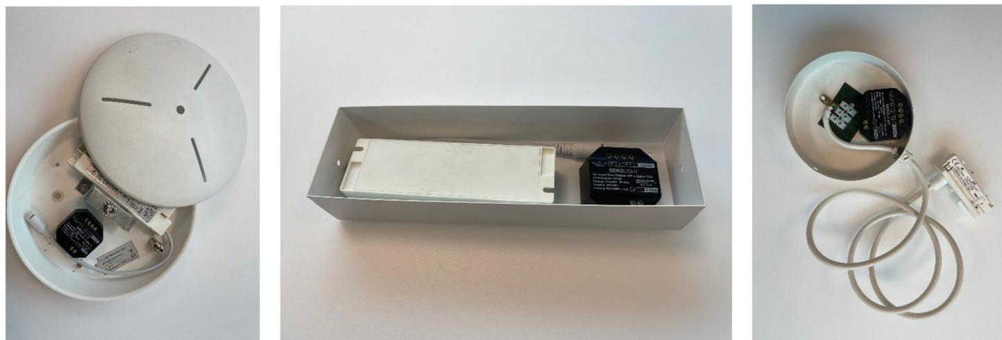
Installation in ceiling canopies (round/angular), directly in luminaires or in the D-ONE 1-phase power feeder(720010/11)
