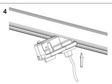
Einsetzen des Adapters in die Stromschiene. / Inserting the adapter into the track.
