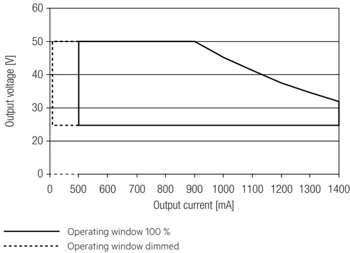
Make sure that the LED Driver is operated within the given window under all operating conditions. Special attention needs to be paid at dimming and DC emergency operation as the forward voltage of the connected LED modules varies with the dimming level, due to the implemented amplitude dimming technology. Coming below the specified minimum output voltage of the LED Driver may cause the device to shut-down. See chapter "6.11 Light level in DC operation" for more information.
