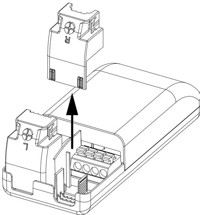
1. Loose strain relief elements from delivery position
