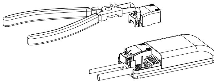
1. Insert release tool device into cut-out, e.g. KNIPEX 46 21 A21 Seeger ring pliers or screwdriver
