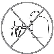
Magnet can only be fastened on the rounded part of the shade.
