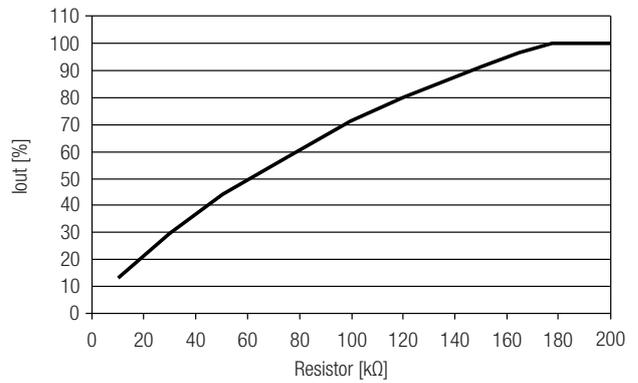
Phase cut dimming curve (depends dimmer)
