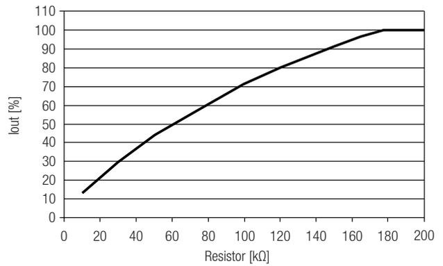
Phase cut dimming curve (depends dimmer)
