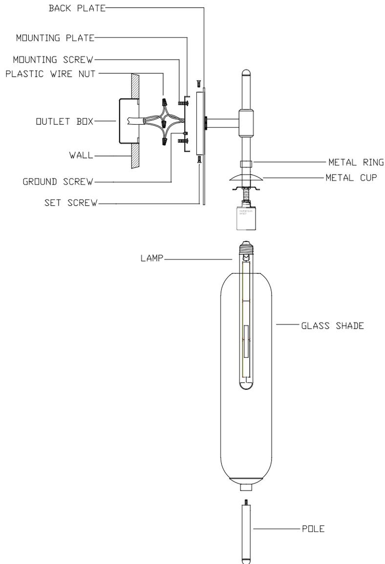
**WIRE NUT/TAPING DIAGRAM**
