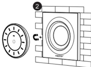
Stick the base well, and the remote control is magnetically attracted to the base
