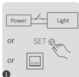
1 Power off 10 seconds and power on again or short press "SET" one time or turn on light via PUSH switch
