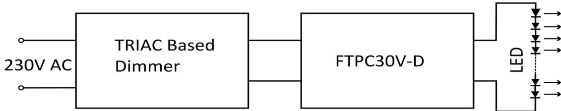
Connection of Dimming operation
