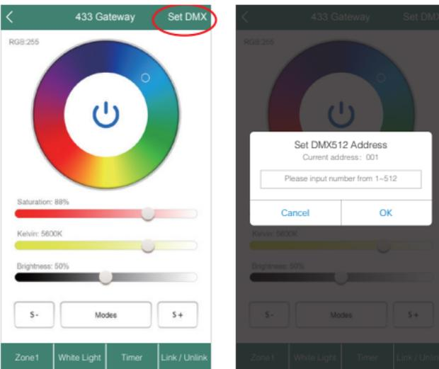
Gateway need to occupy 5 address to control lamp's red,green,blue,warm white and cool white accordingly.
