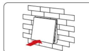
Clicks into the upper side of glass panel on the controller base, then press the lower side slightly to make it clicks into the controller base.
