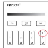
2. Short press any channel "1" 3 times, when linking successfully, DMX512 master indicating lamp will blink 3 times slowly.
