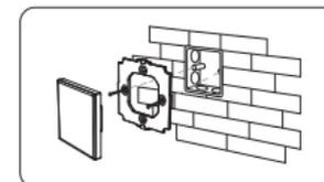
Fix the controller base on the bottom case with screw.
