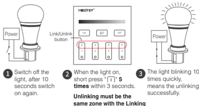
If the light not blink quickly, the unlink failed, pls switch off the light again, and follow the above steps to unlink again.
