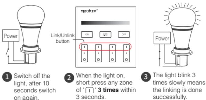
If the light not blink slowly, the linking failed, pls switch off the light again, and follow the above steps again.
