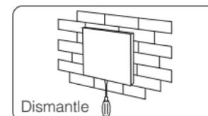
Plug into the below bayonet with a screwdriver, and upwarp screwdriver, then you can dismantle the controller.
