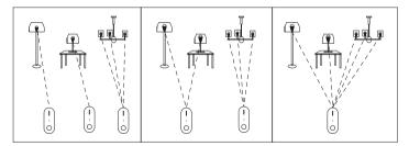
Good to know that one dual white light can connect with up to four different remote controllers, that is 16 unique zones!
